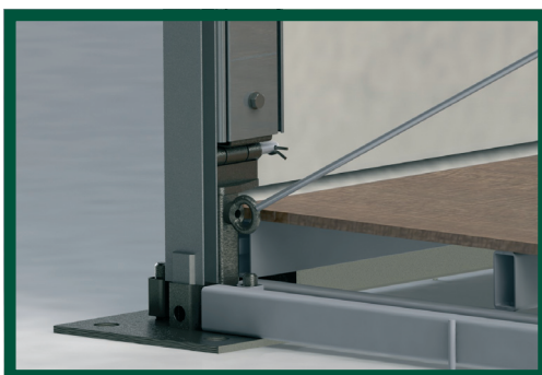
Wind bracing attached to base plate
